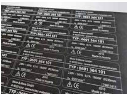
Produce typeplates by directly marking metals
