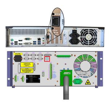
The machine is connected to the Ethernet via a cable connection from the LAN interface on the rear of the PC rack to the LAN interface on the laser rack.
