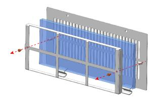
2. Remove both screws and open the cover. Change the filter pad.
