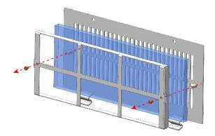
2. Remove both screws and open the cover. Change the filter pad.
