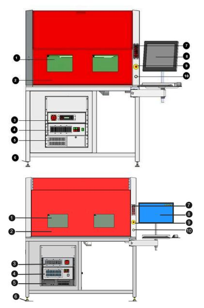
1 Safety glass 2 Safety door 3 Control rack 4 Laser rack 5 Industrial PC 6 Feet (rolls optional) 7 Keypad 8 Monitor, keyboard, mouse 9 Emergency stop button 10 Start button
