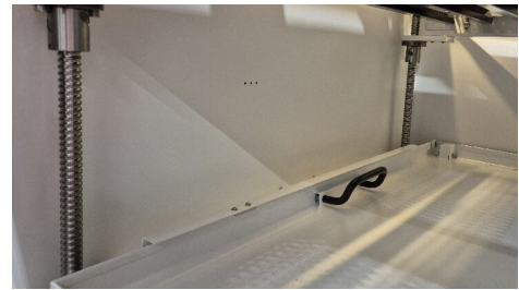
Detail of spindles Z-axis
