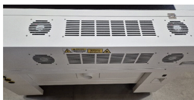
Ventilation grille in the cover of the laser source (closed)
