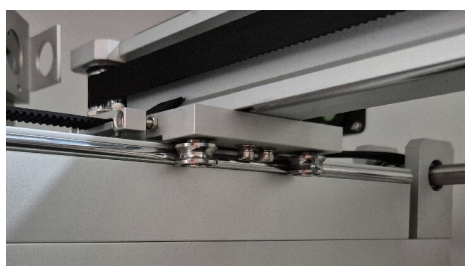
Detail of guide roller with bearing and rails, Y-axis (left)
