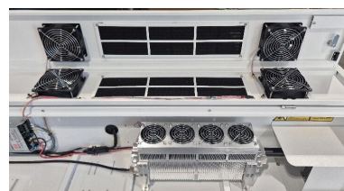
Ventilation grille in the cover of the laser source (open)
