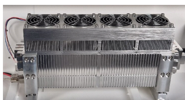
Fan and ventilation grille of the laser source
