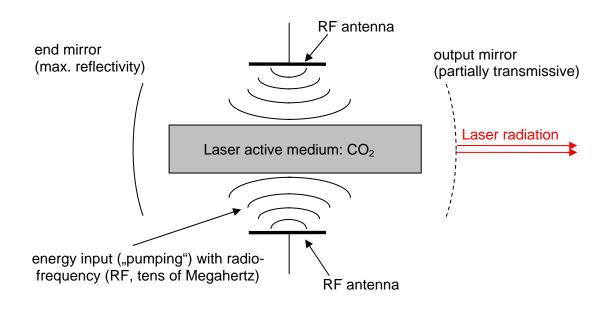
Fig. 1: schematic drawing of a sealed-off CO<sub>2</sub> laser
