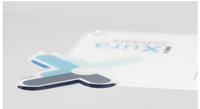
Laser cutting creates crystal-clear cut edges
