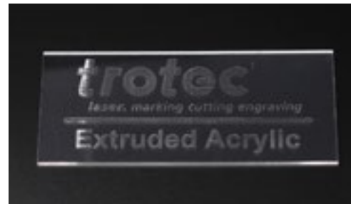
Engraving extruded acrylic will result in little to no contrast
