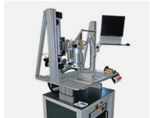
Manual workstation with selective laser shielding
