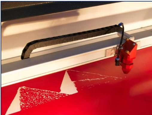
It depends on the material you are using. You should start high on cast acrylic (10 to 20 khz); and start lower on extruded (2 to 5 khz). Decreasing the frequency means there will be less pulses, which results in less energy in the material. This causes:
