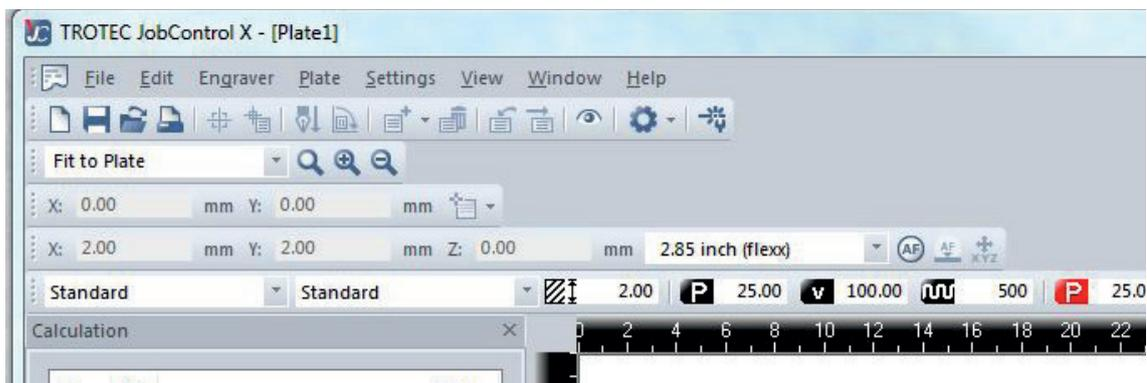
You can change the parameters 'on the fly,' simply by entering the values in the edit line and pressing Enter
