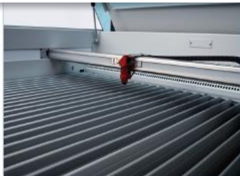
Cutting table with aluminium lamellas for reflection-free cutting
