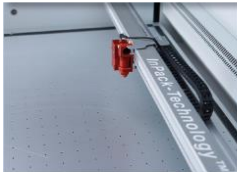
Vacuum table for thin and light materials
