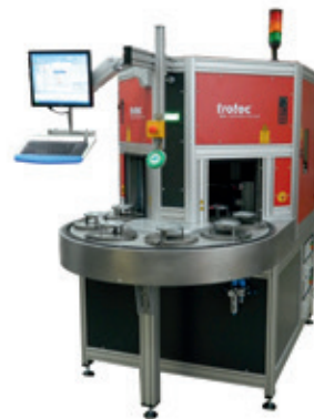
Lid marking using rotary indexing table system
