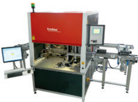
Marking of forceps in laser marking installation with belt rotation system
