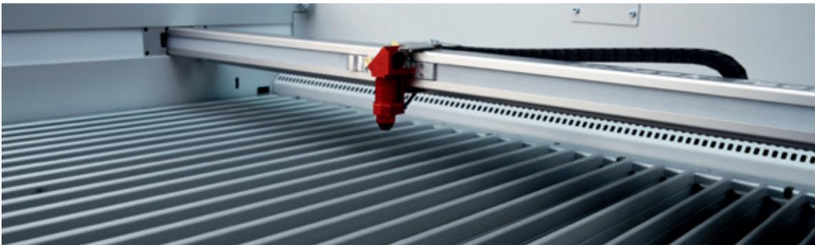
Lamellae can be removed individually and reinserted flexibly
