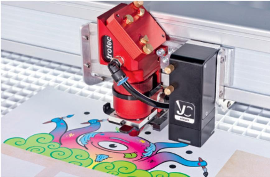
JobControl Vision<sup>®</sup> camera mounted on a Speedy laser head
