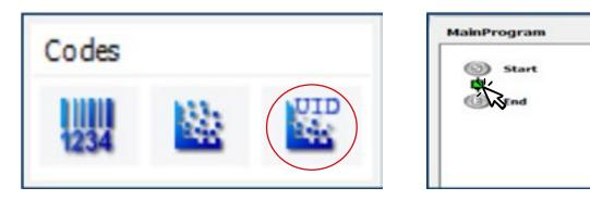
Select UID Datamatrix barcode from the "Codes" section on the left side of the SpeedMark software.
