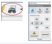
Position the job before starting the marking process. The pilot laser can be used to outline the position of the mark on the work piece. To start press F9 or use the icon in the menu bar.
