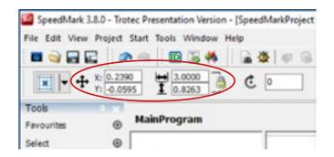
Adjust barcode graphic location by dragging or placing in X-Y coordinates. Adjust the width and or height as needed. Skip to Step 13 on to laser process a 2D barcode.
