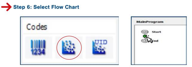
Place the cursor in the flow chart and left click to add it to the flow chart. This will automatically open an import dialogue window as shown on step 7.
