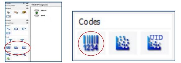
Select 1D (Linear) barcode from the "Codes" section on the left side of the SpeedMark software.
