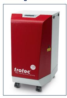
Exhaust plays a huge role in achieving flame polished edges. It is important to have downdraft suction beneath the acrylic to evacuate the gases so they do not become "trapped" in the cut kerf. Without adequate exhaust, a quality cut is not possible. Negative pressure is more important than air flow. The exhaust serves two purposes:
