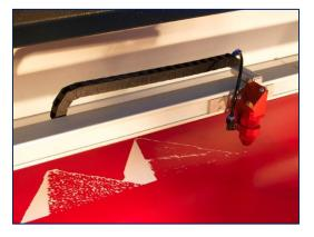
It depends on the material you are using. You should start high on cast acrylic (10 to 20 khz); and start lower on extruded (2 to 5 khz). Decreasing the frequency means there will be less pulses, which results in less energy in the material. This causes:
